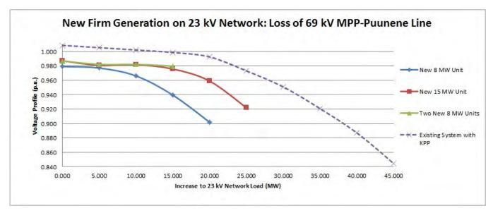
Figure 31: Comparion of P-V characteristics for new firm generation on 23 kV network option for losing the 69 kV MPP-Puunene Line.
