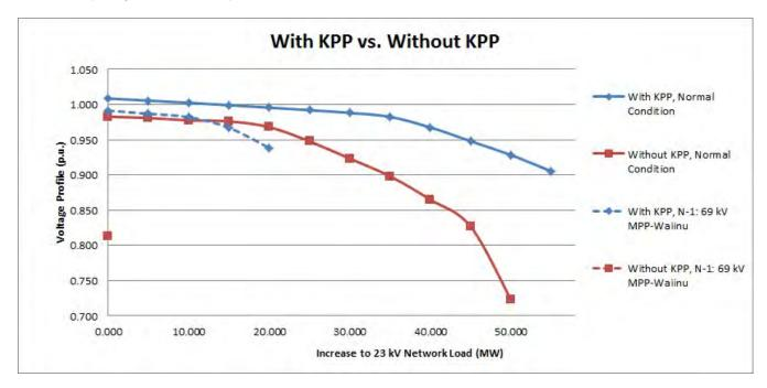
Figure 3: P-V characteristics comparison between system with and without the operation of KPP.
