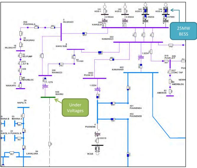
Figure 6: 25MW BESS modeled on the 23kV system improves voltages under N-1 contingency, loss of MPP-Waiinu
