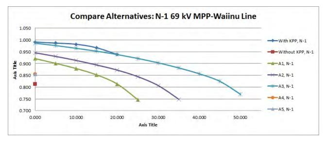
Figure 5: Comparison of P-V characteristics of transmission Alternatives for losing the 69 kV MPP-Waiinu Line. Alternative 1, Alternative 2, Alternative 3, Alternative 4, and Alternative 5 are represented by A1, A2, A3, A4, and A5 respectively.
