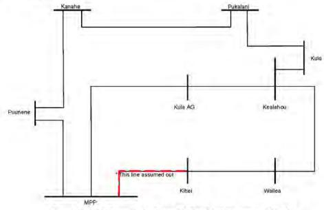
Figure 15: 69 kV Transmission Lines Feeding South/Up-country Maui Area
