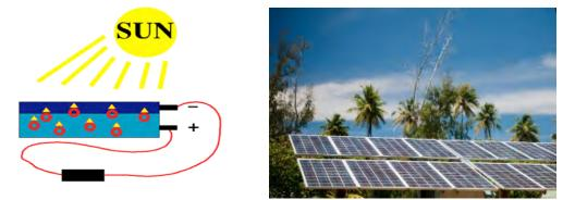
Figure G-3. Schematic of a Photovoltaic (PV) Cell and an Array of PV Panels
