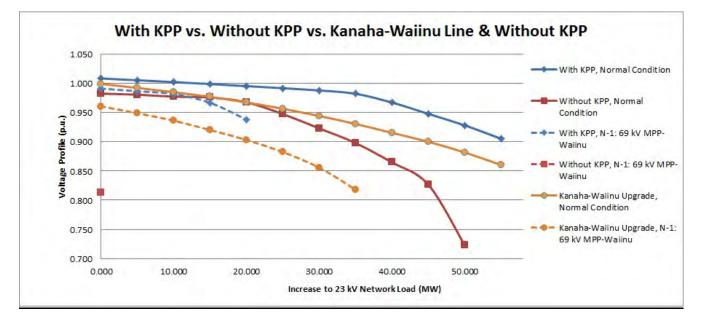
Figure 8: P-V characteristic comparison of the Maui system operating with and without KPP and the system operating without KPP under the scenario that Combo 4 is implemented for the normal condition and most severe N-1 contingency.
