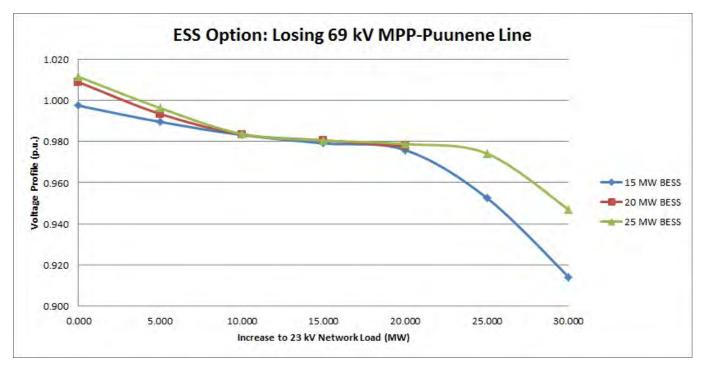
Figure 37 Comparison of P-V characteristics of various BESS options for losing the 69 kV MPP-Puunene Line.
