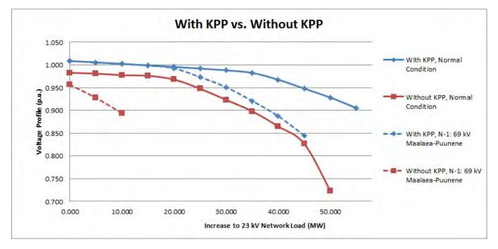
Figure 19: P-V characteristics of existing systen with and without KPP for losing the 69 kV MPP-Puunene Line.
