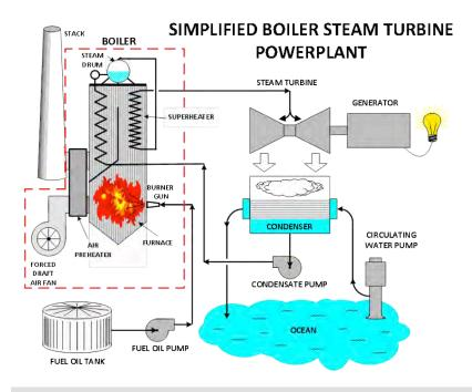
Figure G-10. Simplified Boiler Steam Turbine
