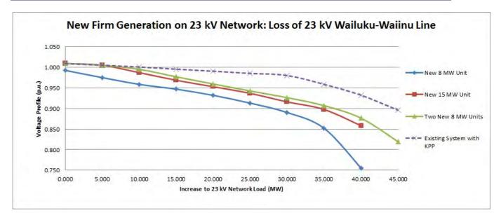
Figure 32: Comparion of P-V characteristics for new firm generation on 23 kV network option for losing the 23 kV Wailuku-Waiinu Line.
