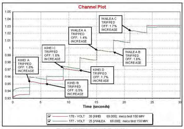
Figure 10: 150 MW Case Manually Shed Load
