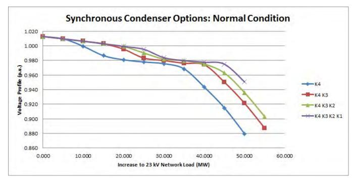
Figure 9: P-V characteristic comparison of different scenarios of KPP units converted to synchronous condensers for the normal condition.
