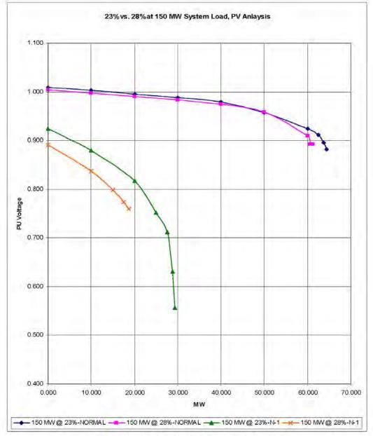
Figure 5: 23% vs. 28% of 150 MW System Load, PV Analysis
