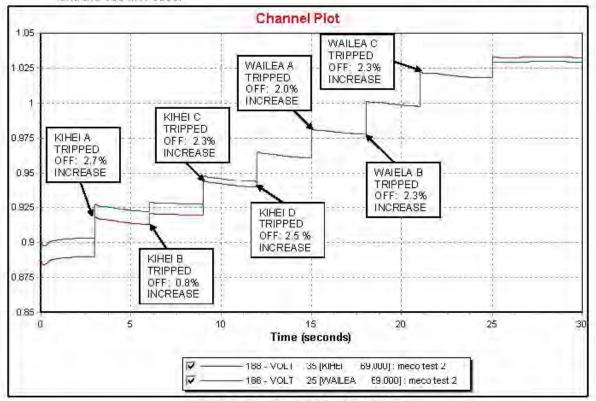
By using dynamic studies to shed loads in the South Maui area, the amount of load needed to be shed per 1% increase in voltage can be calculated and averaged to approximately 3,3MVA. The following plots and tables show this for the Peak Basecase and the 150 MW case.
