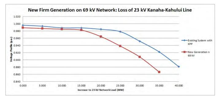
Figure 33: Comparison of P-V characteristics of new firm generation on 69 kV network for losing the 23 kV Kanaha-Kahului Line.
