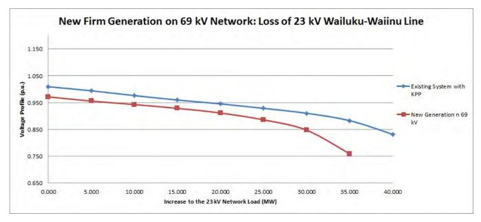
Figure 35; Comparison of P-V characteristics of new firm generation on 69 kV network for losing the 23 kV Wailuku-Waiinu Line.
