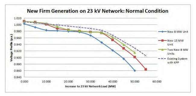
Figure 11: P-V characteristic comparison of different scenarios of new generation of various capacities on the 23 kV network and the existing system for the normal condition.
