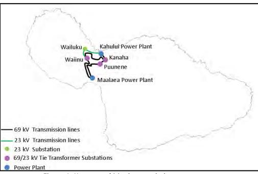
Figure 1: Key central Maui transmission components
