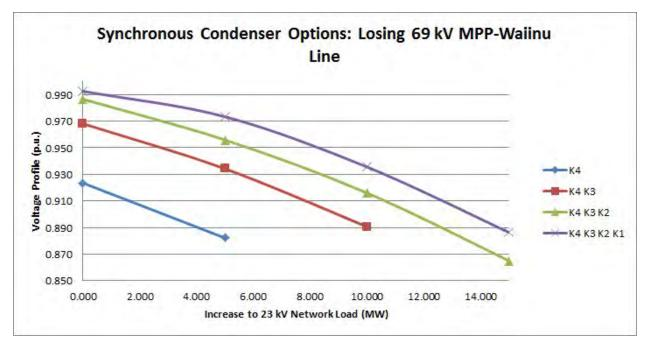
Figure 10: P-V characteristic comparison of different scenarios of KPP units converted to synchronous condensers for the most severe N-1 contingency event.
