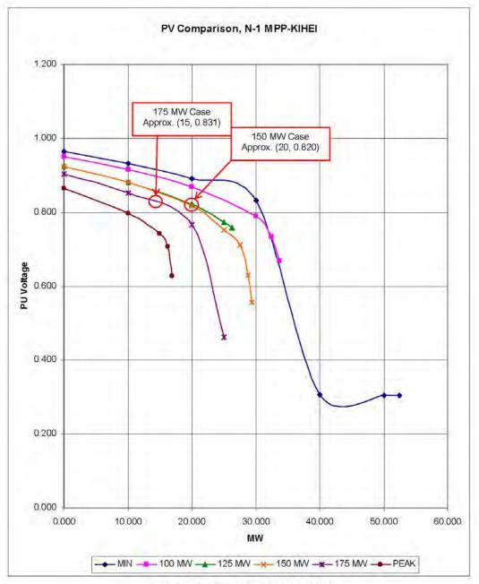
Figure 2: PV Comparison, N-1 MPP to Kihei
