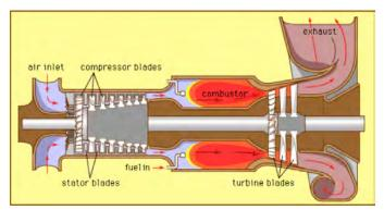
Figure G-7. Gas Turbine Engine
