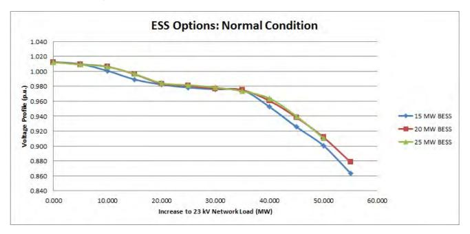
Figure 14: Comparison of P-V characteristics of various sized BESS for the normal condition.
