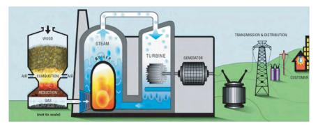
Figure G-11. Biomass Gasification
