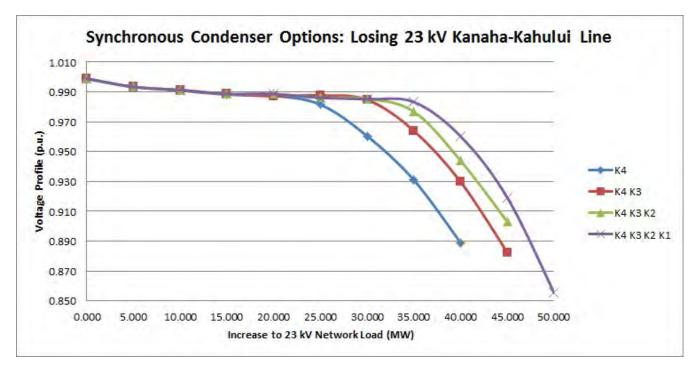
Figure 27: Comparison of P-V characteristics of synchronous condenser options for losing the 23 kV Kanaha-Kahului Line.
