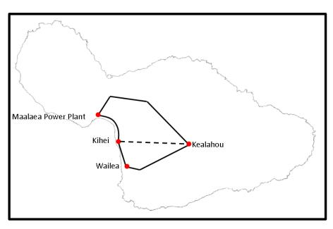
Figure 9: South Maui transmission system with Kamalii Substation and Maalaea-Kamalii 69kV transmission line
