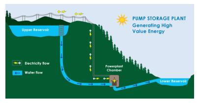
Figure G-6. Pumped Storage Hydroelectricity Plant
