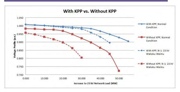
Figure 20: P-V characteristics of existing systen with and without KPP for losing 23 kV Wailuku-Waiinu Line.
