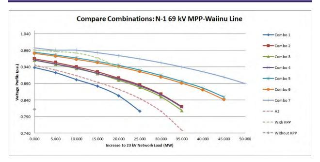
Figure 7: Comparison of P-V characteristics of tranmission Combinations for losing the 69 kV MPP-Waiinu Line. Combination 1, Combination 2, Combination 3, Combination 4, Combination 5, Combination 6, Combination 7, and Alternative 2 are represented by Combo 1, Combo 2, Combo 3, Combo 4, Combo 5, Combo 6, Combo 7, and A2 respectively.
