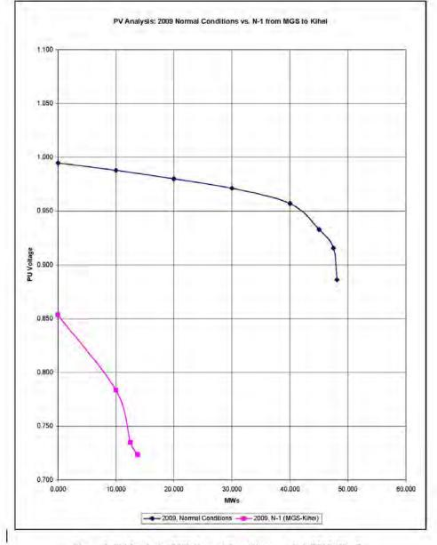
Figure 2: PV Analysis, 2009 Normal Conditions vs. N-1 (MGS-Kihei)
