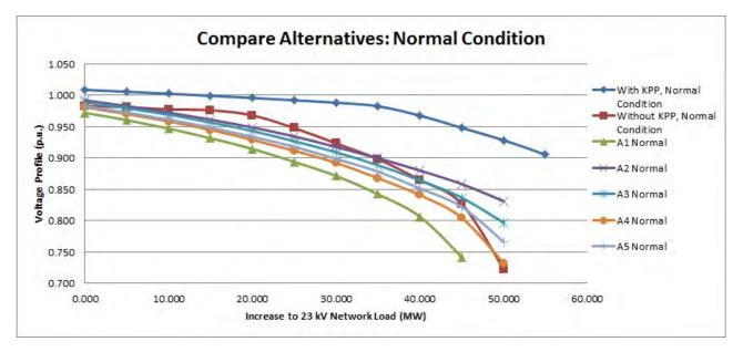
Figure 4: Comparison of P-V characteristics of transmission Alternatives for the normal condition. Alternative 1, Alternative 2, Alternative 3, Alternative 4, and Alternative 5 are represented by A1, A2, A3, A4, and A5 respectively.
