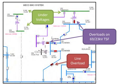
Figure 2: 69kV system current conditions for 2019 under N-1 contingency, loss of MPP-Waiinu
