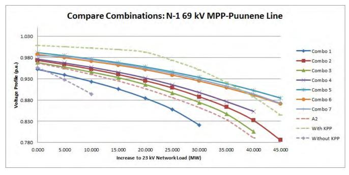
Figure 25 Comparison of P-V characteristics of tranmission Combinations for losing the 69 kV MPP-Puunene Line.
