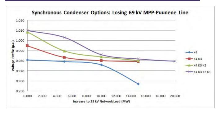
Figure 28: Comparison of P-V characteristics of synchronous condenser options for losing the 69 kV MPP-Puunene Line.
