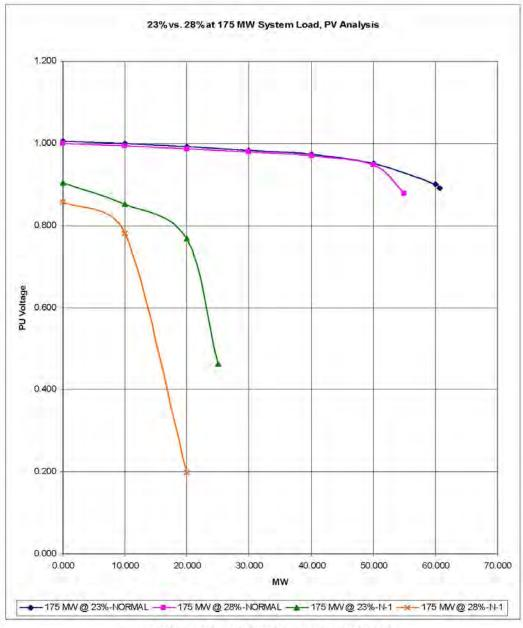
Figure 6: 23% vs. 28% of 175 MW System Load, PV Analysis
