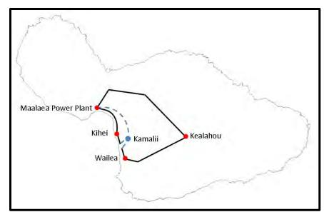
Figure 4: South Maui transmission system with Kamalii Substation and Maalaea-Kamalii 69kV transmission line
