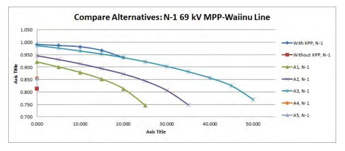
Figure 5: Comparison of P-V characteristics of transmission Alternatives for losing the 69 kV MPP-Waiinu Line. Alternative 1, Alternative 2, Alternative 3, Alternative 4, and Alternative 5 are represented by A1, A2, A3, A4, and A5 respectively.
