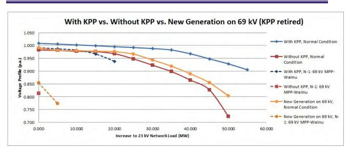
Figure 13: P-V characteristic comparison of the scenario of new generation on the 69 kV network, the existing system with KPP, and the existing system without KPP for the normal condition and most severe N-1 contingency event.
