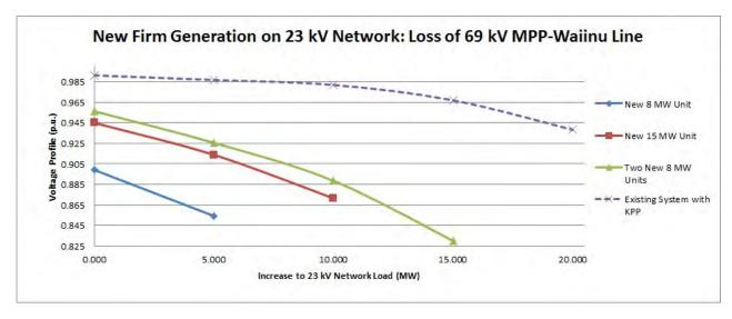
Figure 12: P-V characteristic comparison of different scenarios of new generation of various capacities on the 23 kV network and the existing system for the most severe N-1 contingency event.
