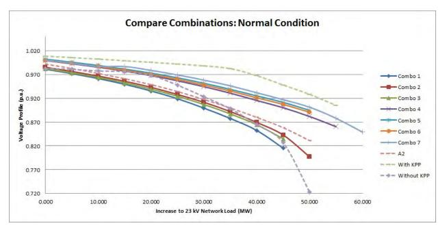
Figure 6: Comparison of P-V characteristics of tranmission Combinations for the normal condition. Combination 1, Combination 2, Combination 3, Combination 4, Combination 5, Combination 6, Combination 7, and Alternative 2 are represented by Combo 1, Combo 2, Combo 3, Combo 4, Combo 5, Combo 6, Combo 7, and A2 respectively.
