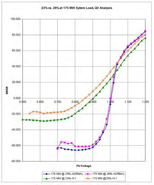
Figure 8: 23% vs. 28% of 175 MW System Load, QV Analysis NOTE: N-1 condition in figure above is with the line from MPP to Kihei out.
