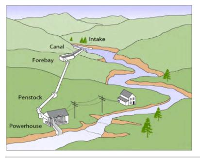
Figure G-5. Run-of-River Hydroelectric Plant
