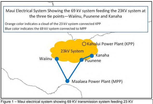
transmission system at three tie points - Waiinu, Puunene, and Kanaha
