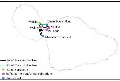
Figure 1: Key central Maui transmission components
