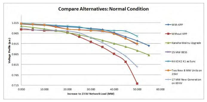
Figure 16: Comparison of P-V characteristics of various NTA options against the Kanaha-Waiinu upgrade and existing system with and without operation of KPP for the normal condition.
