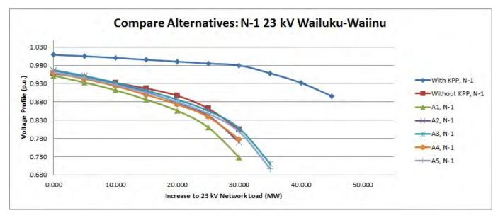
Figure 23; Comparison of P-V characteristics of transmission Alternatives for losing the 23 kV Wailuku-Waiinu Line.
