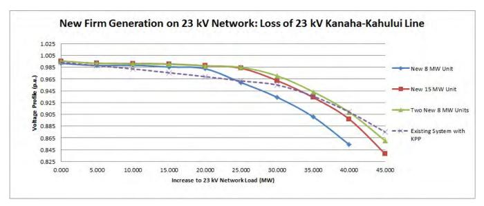
Figure 30: Comparion of P-V characteristics for new firm generation on 23 kV network option for losing the 23 kV Kanaha-Kahului Line.
