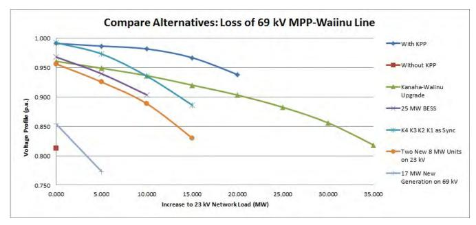
Figure 17: Comparison of P-V characteristics of various NTA options against the Kanaha-Waiinu upgrade and existing system with and without operation of KPP for the most severe N-1 contingency.
