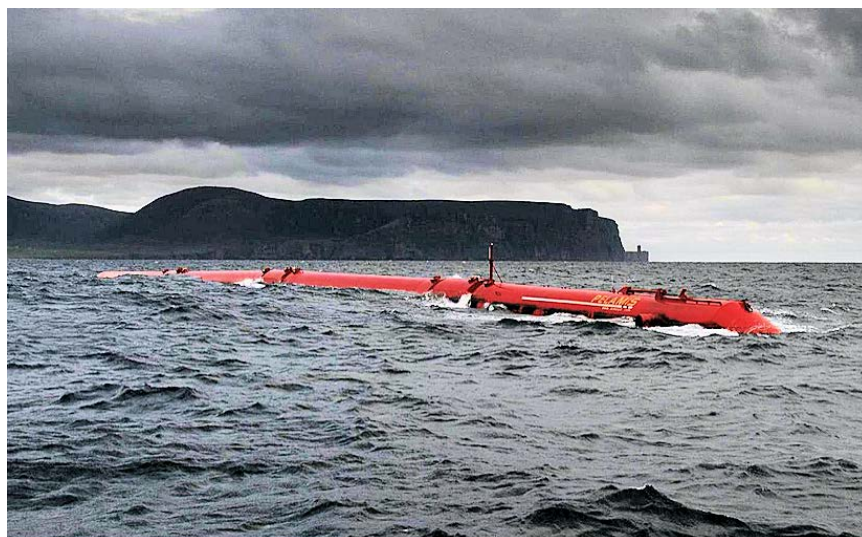
Figure H-21. Pelamis Wave Energy Converter at the European Marine Energy Test Centre, 2008
