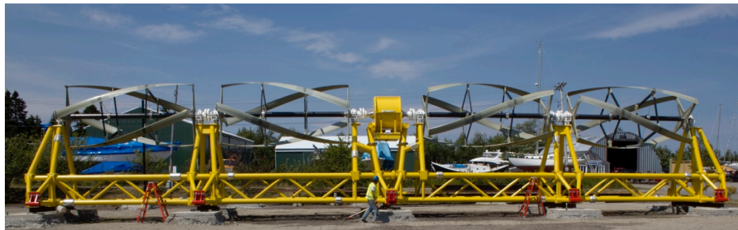
Figure H-19. ORPC TidGen Tidal Generator
