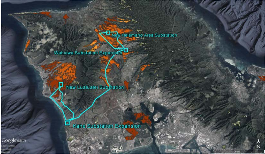
Figure N-49. Approximate 138 kV Transmission System Expansion to Accommodate Grid-Scale PV in High-Potential Areas
