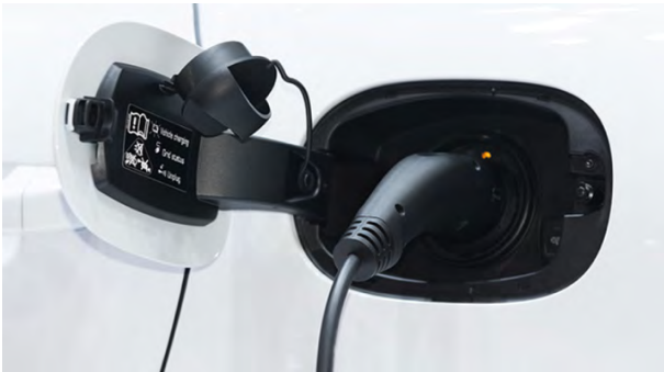
Figure 2-7. Level 2 Electric Vehicle e-Charger
